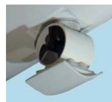
Leaves smooth hull lines when retracted and achieves ideal immersion depth when deployed
